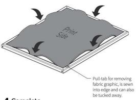
**3** Use downward pressure to insert the remaining edge, working out from the center toward each end.
