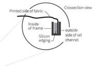
**2** Insert fabric edge only at the center of each channel, pushing directly downward.
